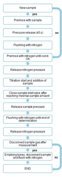
Figure 1: Method sequence of a water determination in gas (I or g)
