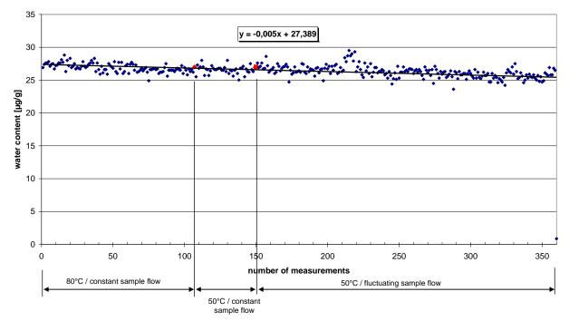
Figure 2: Measured water contents during long-term test
