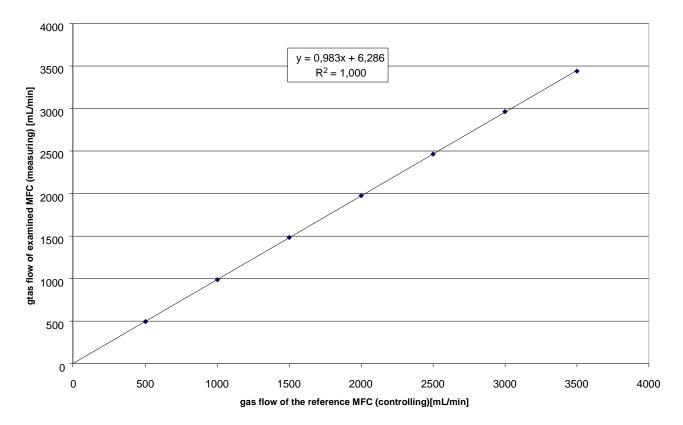
Figure 7: Reference flow versus measured flow - after long-term test
