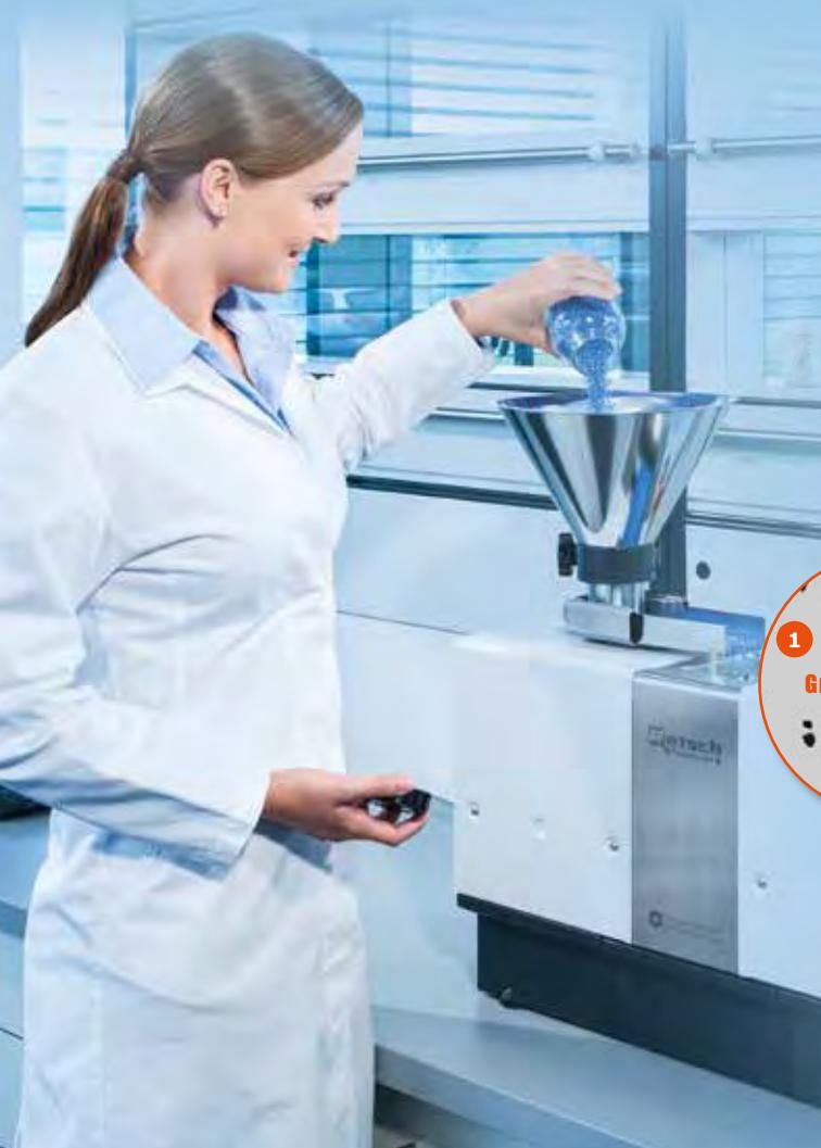
DIA analyzes the shadow projections of particles. Both the CAMSIZER P4 and CAMSIZER XT transform grayscale images through a multistep algorithm into binary images to determine the exact outlines. All size and shape parameters are measured on this basis. The values of the single measurements are assigned to 10,000 size classes during the measurement, providing an extremely high resolution.
