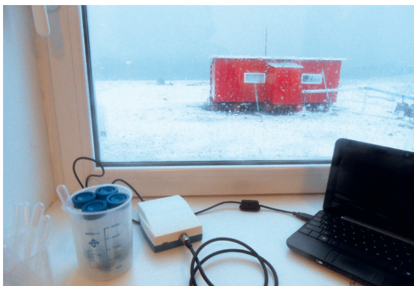
Figure 5 (top). To determine the oxidation potentials of the dyes I had extracted, I used an experimental setup that consisted only of the 400 \mu Stat potentiostat and a laptop. Figure 6 (left). Here I am measuring the oxidation potential of a dye using the \mu Stat 400 from DropSens.
