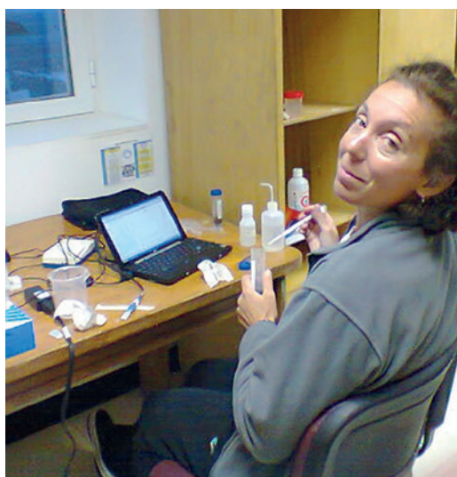
Figure 5 (top). To determine the oxidation potentials of the dyes I had extracted, I used an experimental setup that consisted only of the 400 \mu Stat potentiostat and a laptop. Figure 6 (left). Here I am measuring the oxidation potential of a dye using the \mu Stat 400 from DropSens.
