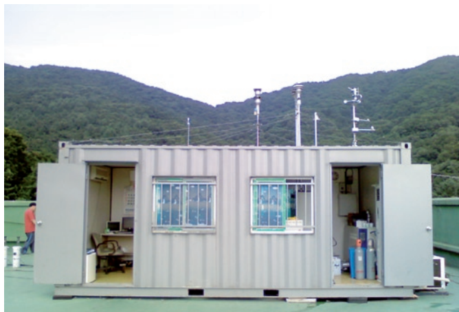
Measuring station for air quality monitoring: among the analyzers installed in this portable building is a MARGA system, which can be operated fully automatically over an extended period of time.
