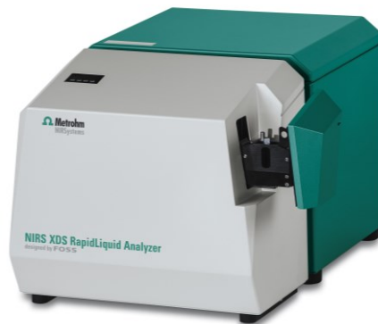
Fig. 1: A NIRS XDS RapidLiquid Analyzer equipped with 4 mm NIRS quartz cuvette with a screw top were used to generate the spectral data in true transmission mode.
