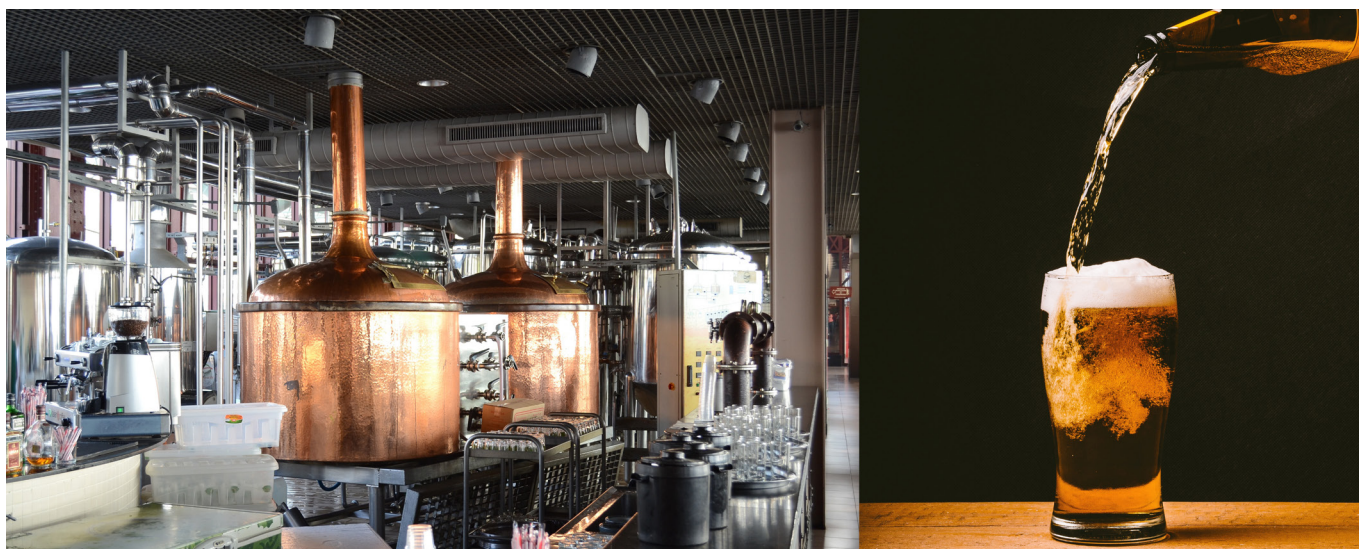
Large copper boiling kettles utilized at a commercial brewery along with the final product.
