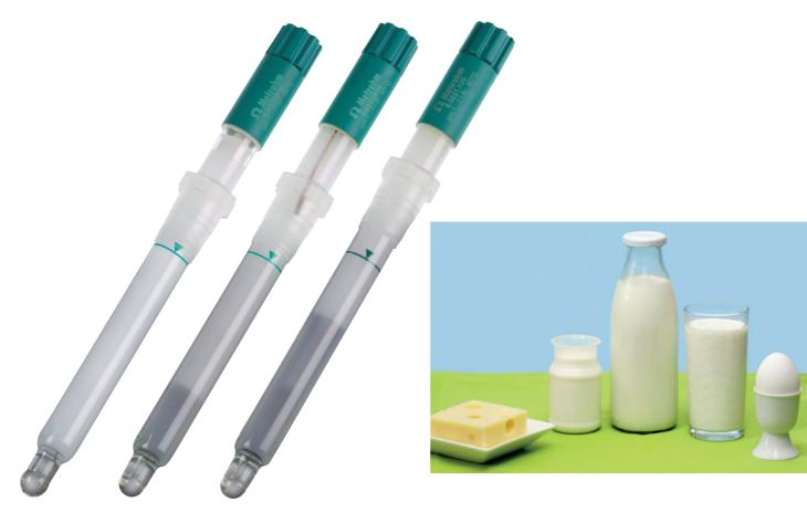
Still within the permissible operating range: The decolorized zone of the gel gradually spreads up to the mark with use.
