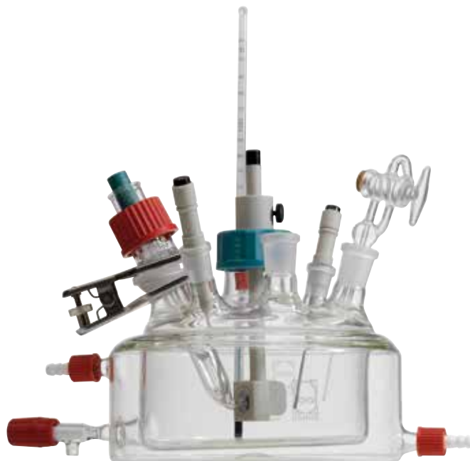
The Autolab PGSTAT204 and corrosion cell for corrosion research
