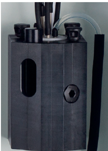
(L) Thermostated cuvette module at the heart of the 2029 Process Photometer. (R) Drift-controlled measured value acceptance.
