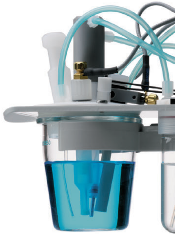
Cell with electrodes for CVS analysis of a Cu bath
