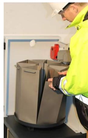
The first part sample of 6 liters is again fed to the hopper and reduced to the desired number of part samples with the module for discontinuous operation, for example 10 samples of 600 ml (fig. 7).
