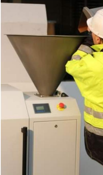
Both division processes don't take longer than 10 minutes and not only offer considerable time saving but also consistent working conditions resulting in reliable sampling results; this is a clear advantage over manual sample division or using a sample splitter. Another pro: the PT 600 XL is quickly and easily cleaned because all parts coming into contact with the sample can be easily removed.
