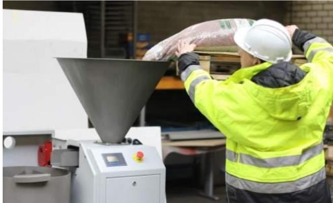
Fig. 4: Up to 60 l of sample material can be fed to the hopper of the PT 600 XL
